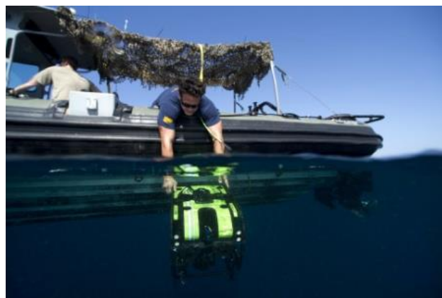
Figure 1: An Explosive Ordnance Technician, Task Group 56.1, deploys an ROV in the Arabian Gulf. (Courtesy of the Defense Video & Imagery Distribution System)
